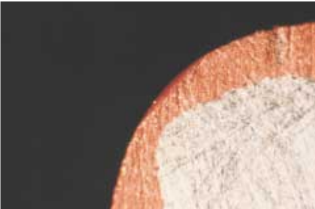
Figure 4. Cross-section showing reduction in coating thickness at a corner (image courtesy of Steel Protection Consultancy)
