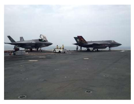
BF-1, heavily instrumented for the trials, was down owing to a faulty cooling fan in the engine nacelle; this was repaired and the aircraft conducted flights later in the day after we departed the ship. BF-5, a production representative model, was having trouble with its thermal management subsystem.
